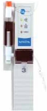
Figure 1 - 2: The Air Detector/Automatic Clamp, which is a standard fitting for H-1200, can be retrofitted to earlier models. The model shown here is a H-31B, developed from the earlier SA-1000 and H-30 models. (see section 8 for details)
