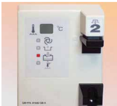
Figure 1 - 6: Alarm - Recirculating Solution Level Low
