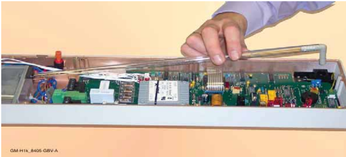
Figure 4 - 2: Once the elbow is released, the tube can be withdrawn gently from the reservoir tank.
