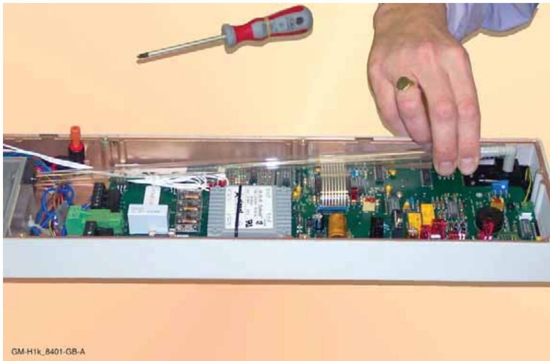
Figure 4 - 1: A sharp upward tug will usually disconnect the Return Pipe.
